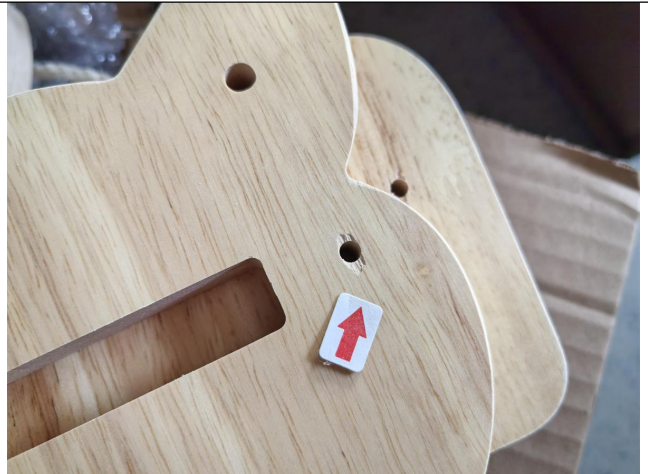
Punch hole of the template is chipped100%(Remark 3)
