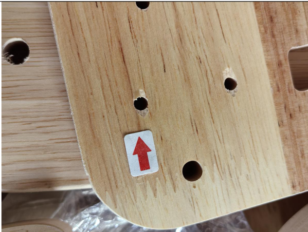
Punch hole of the template is chipped100%(Remark 3)
