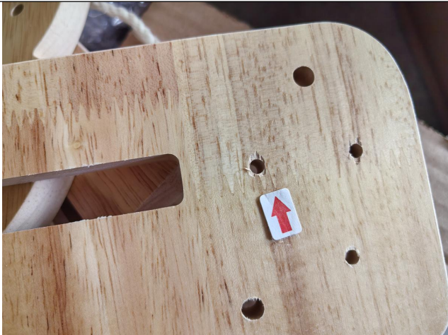
Punch hole of the template is chipped100%(Remark 3)
