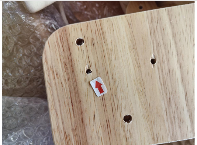
Punch hole of the template is chipped100%(Remark 3)
