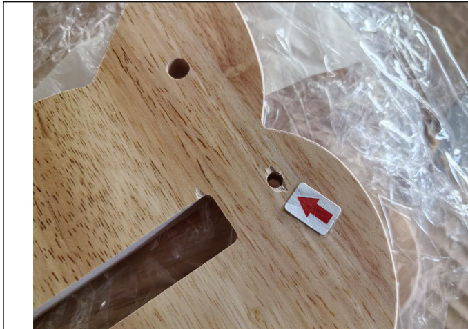
Punch hole of the template is chipped100%(Remark 3)
