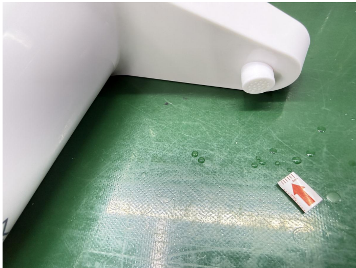
Water inside the faucet not be drained off
